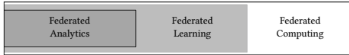
Fig. 1. Intersection of definitions for FC, FL, and FA. FC consists of FL and FA, whereas FL systems can contain FA characteristics. FA is a subset of FL and FL is a subset of FC.
